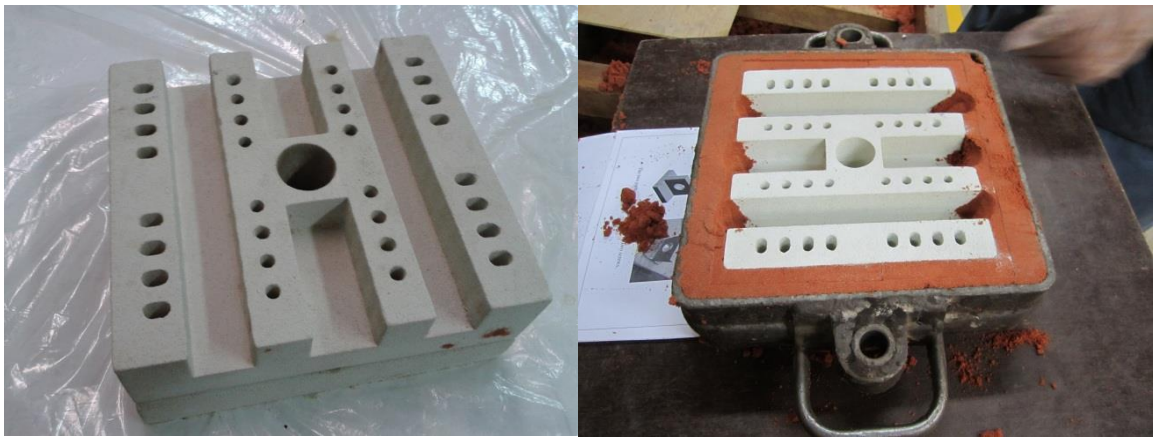
Figure 21 (a) Optimized 3D Printed Ceramic Mold Design (b) 3D Printed Ceramic Mold for casting
