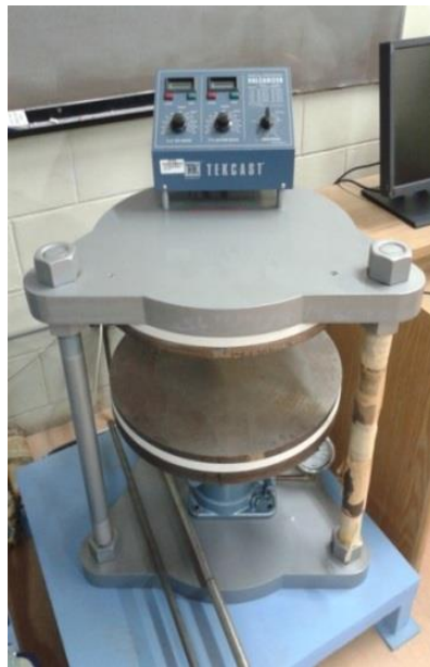
Figure 25 Mold vulcanizing setup including the TEKCAST vulcanizer machine with press
