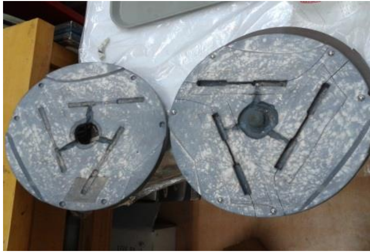
Figure 49 Spin cast Mold for casting the Dumbbell shaped Tensile Test Specimens
