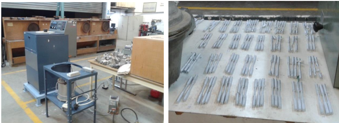
Figure 29 (a) Spin Casting Setup, (b) Spin Cast sample sets casted at varying Parameters
