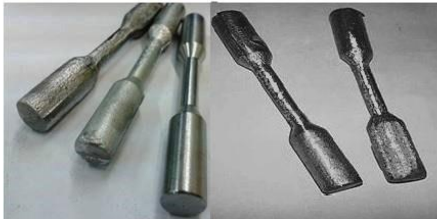
Figure 66 Surface Finish of casted samples from left to right (sand cast, spin cast, machined standard sample, plaster mold cast, 3D printed ceramic mold cast)
