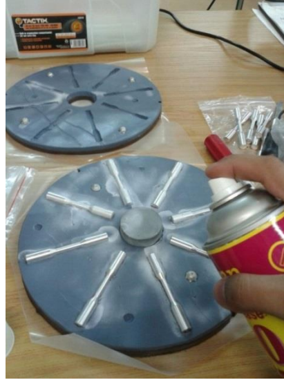
Figure 28 Spin Casting silicon mold
