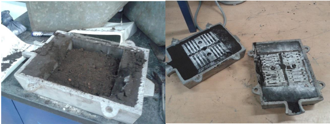
Figure 18 (a) Preparation of Sand mold (b) Sand mold halves ready for casting
