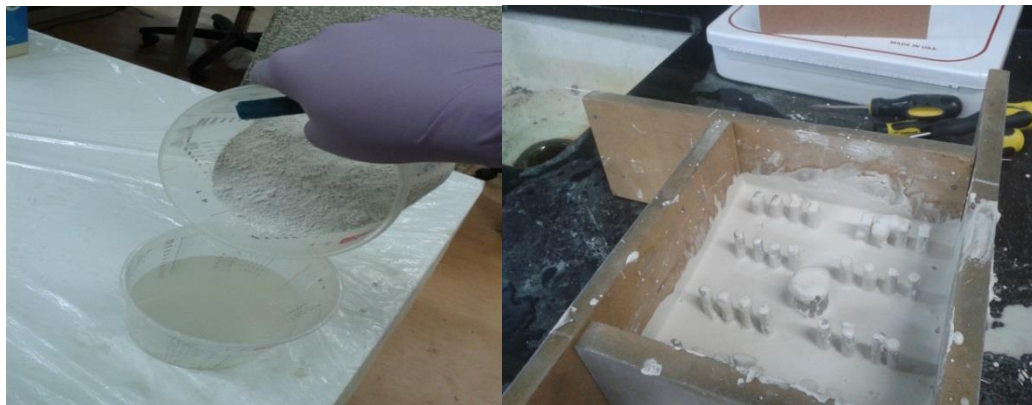
Figure 16 (a) Mixing plaster into the water to make slurry (b) Curing of plaster mold
